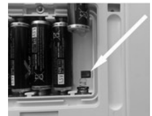
Picture 2: Tune volume of internal loudspeaker
